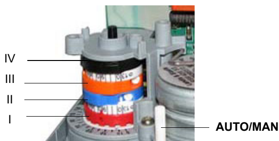
Siemens SQN72.2A4Ax (high-low flame burners)
