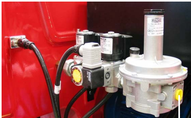
connection to the gas supply network - 1/2"
