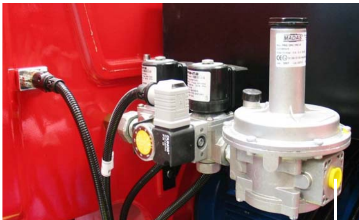
connection to the gas supply network - 1/2"
