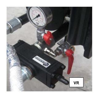
6 Set the atomisation air according to the data in the nozze diagram attached, by means of the RB knob (see picture).
