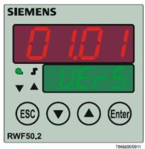
The software version is shown by pushing  $\mathbf{Enter} + \mathbf{UP} \ \mathbf{arrow}$  on the upper display
