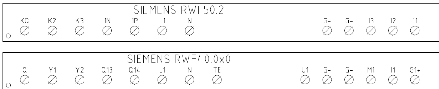
Matches terminals between RWF50.2 and RWF40.0x0
